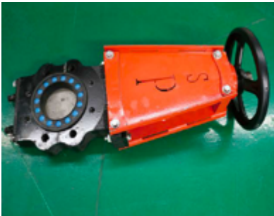
Cut off Valve
